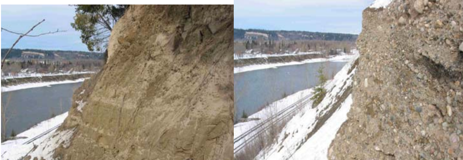
Figure 10: Close-up of the upper sand layer underlying forest floor (left) and underlying lower layers of gravel (right).
