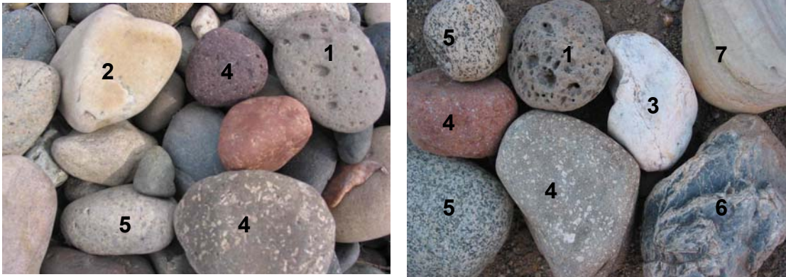
Figure 11. Different types of pebbles in gravel. 1, volcanic lava with gas bubbles. 2, quartzite. 3, quartz. 4, volcanic lava. 5, granitic rock. 6, chert. 7, mudstone.
